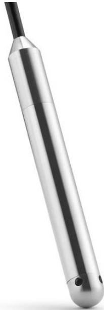
Level transmitter with submersible probe in stainless steel for level measurement in vessels where pressure connection in the bottom of the vessel is not possible or desirable. For example pump pits, reservoirs or plastic tanks.
